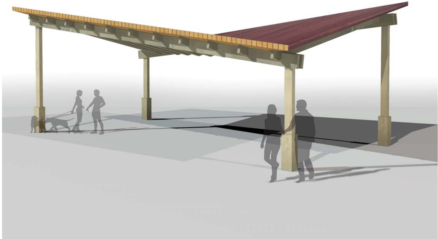
Prefabricated 25' x 60' steel structure with standing seam metal roof and tongue and groove wood finish below. Rain chain to connect to stormwater feature.
