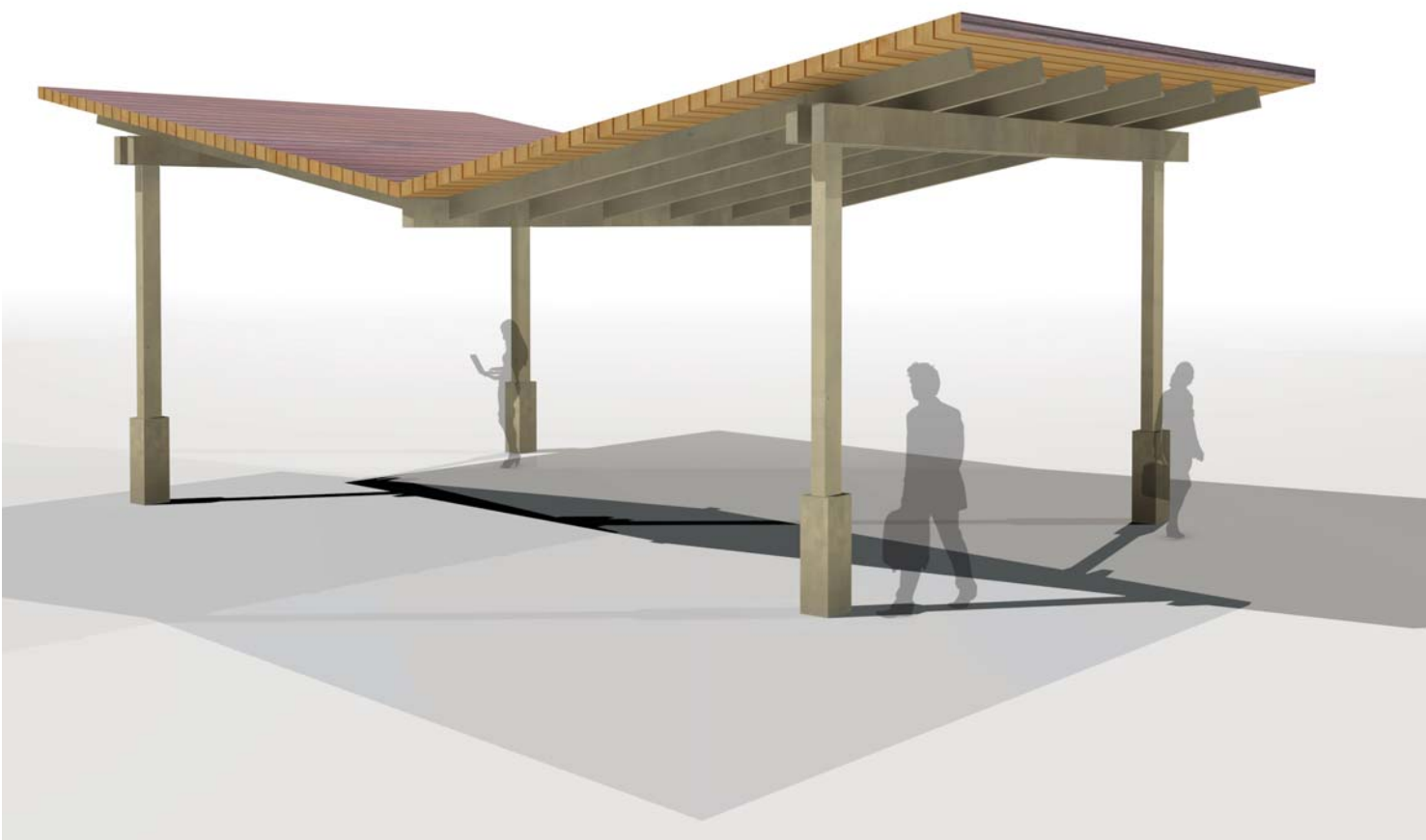
Prefabricated 25' x 45' steel structure with standing seam metal roof and tongue and groove wood finish below. Rain chain to connect to basin.
