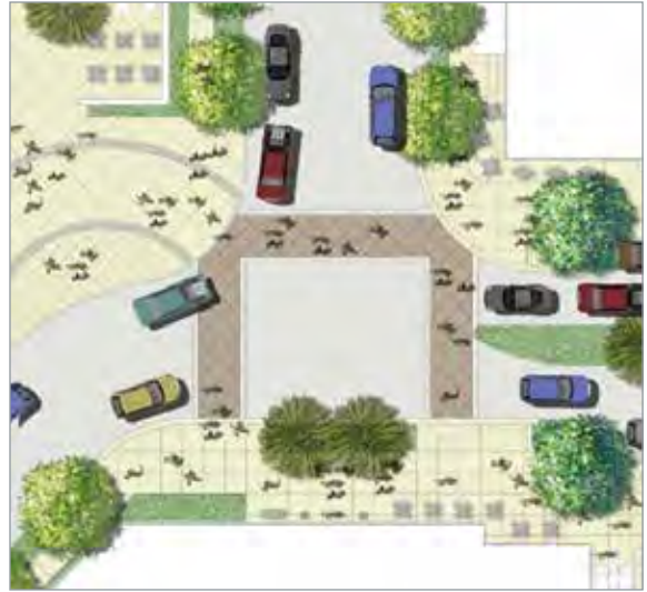
Figure 3.1b Conceptual Plan of Crosswalk Enlargement
