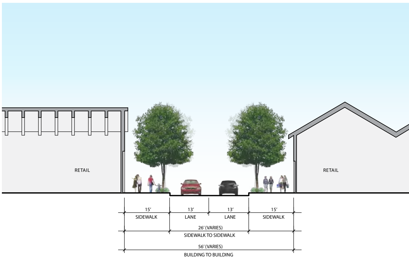
Figure 3.2d Private Driveway “C” Section
